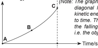
(Note: The graph is a curve and not a straight diagonal line because the change in kinetic energy is not directly proportional to time. The rate of change of speed of the falling object increases over time i.e. the object accelerates as it falls.)
